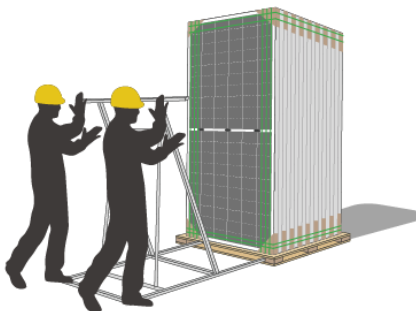
4) Place the stand supporter from the glass or backsheet side.
