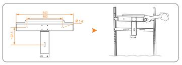
Step 2 Mount the inverter on the rear panel and tighten the inverter with the rear panel by locking screws at the bottom of the inverter.
