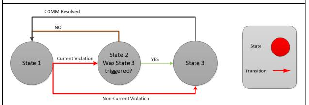
Communication and power supply failures between **Components** and **Devices**. Please document here compliance with EREC G100 section 5.5.
