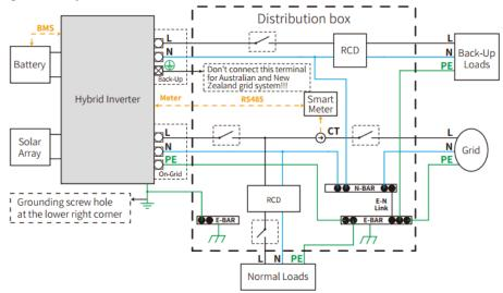
Example for grid systems without special requirements on electrical wiring connection. (The back-up PE line and earthing bar must be grounded properly and effectively. Otherwise the back-up function may be abnormal when the grid fails.)
