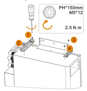
2. Attach the inverter to the mounting bracket. Mount the supporting bracket at the bottom of the inverter.
