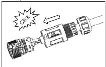
3 Plug the Backup connector into the socket for the Backup connection and screw tight, when doing so, align the Backup connector so that the key on the inverter Backup socket is inserted into the keyway on the AC connector bush.
