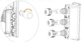
Unscrew the nut of cable gland and take out the rubber cylinders.
