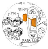
2. Tighten the Wi-Fi module onto the inverter with screw M4\*10 (X2) (Tool: PH2 screwdriver,torque: 2.0 Nm).
